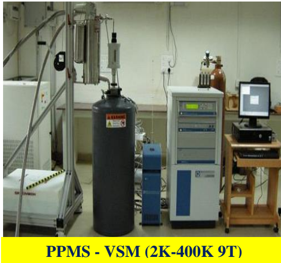
Figure 17. Photograph of a Physical Property Measurement system - Vibrating Sample Magnetometer (Quantum Design, USA) setup. Figure. 18. a) Resistivity sample puck, b) Front view of resistivity sample puck, c) Rear view of the sample puck, and d) Schematic representation of a four-probe method.
